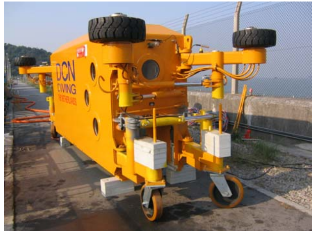
An SCH. The black drive wheels operate against the culvert walls.
