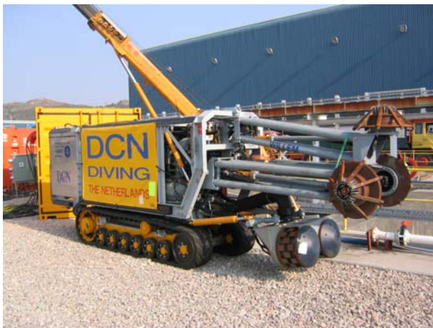
An ROCM with three computer controlled cleaning heads and a floor level grinder and crusher,
