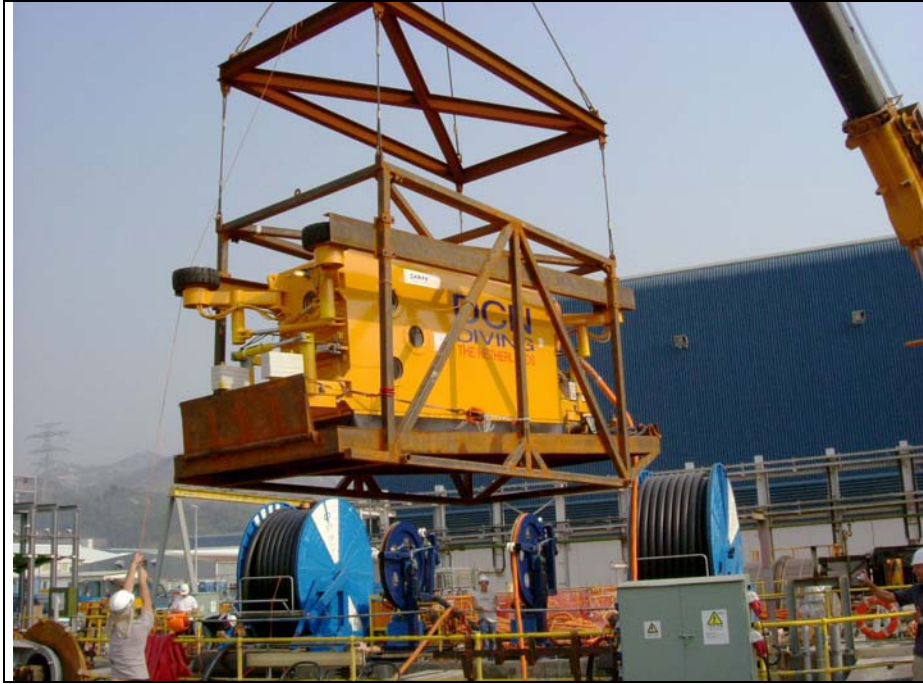
Deployment of the habitat inside a handling frame.
